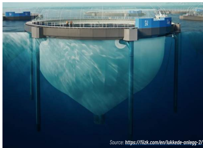
Figure 1: Protectus flexible containment tank.
