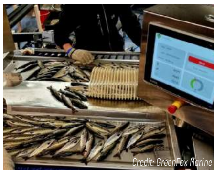
The gender-sorting machine in use at Mowi
