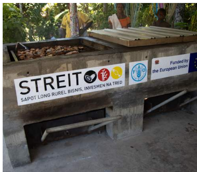
The final product in the Papua New Guinea site: the FTT kiln, variations of which have been constructed in small-scale fish smoking and drying operations across over 20 developing nations
