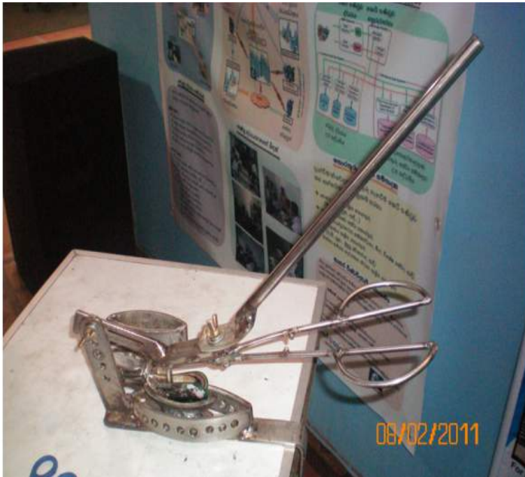
A patented knife has been invented to help the gleaners to process the mussels safely
